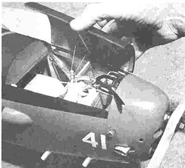
Inverted Torp gives no running problems, reports CH, because of choke installation. Motor is mounted on an adapter plate.
