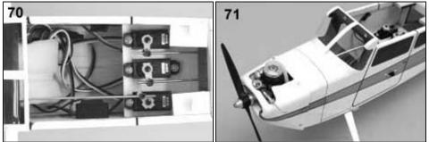
71. Install the windshield on the model. First glue the top rear edge to the top of F-5. When this glue is dry, use small strips of masking tape to hold the bottom corners in position and carefully glue the remaining edges of the windshield to the model.
