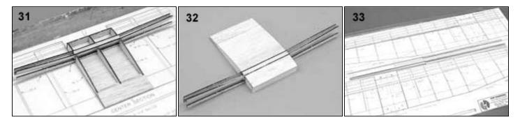
34. Trim the ends of the 1/16 x 1 trailing edges (where they meet at W-7) to the angles shown on the plan. Glue the trailing edges together over the plan. When the glue is dry, trim the outer piece to match the plan. Assemble the three remaining trailing edges as you did the first.
