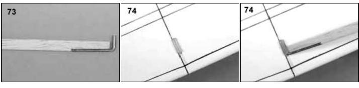
75. Mount the wing on the model. Attach the strut to one of the wings by sliding the wire into the tube. Now swing the strut against the fuselage side and cut it off so that there is about 1/8 between the end of the strut and the tube on the fuselage. Now attach the lower strut wire to the strut. Build the other strut and finish them with covering material.
