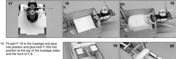
20. Glue parts F-10, F-15 and F-16 into position at the nose of the model. Now glue the 3/16 sq. strip into position between F-7 and F-16.
