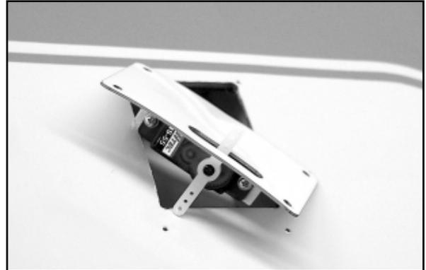
The servos/servo hatches are now installed into each wing panel and their mounting screws secured. Turn off the airborne radio system and disconnect the switch and the Y-harness from the receiver and the battery from the switch. Turn off your transmitter.
