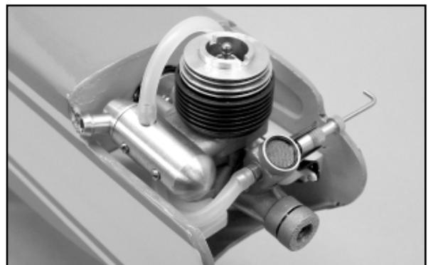
Re-install the output arm retaining screw in the throttle servo. Reassemble the muffler and needle valve back onto the engine. Trim the silicon fuel tubes to fit onto the carburetor and muffler pressure nipple. Be sure to leave enough slack to easily grip these tubes for fueling purposes.
