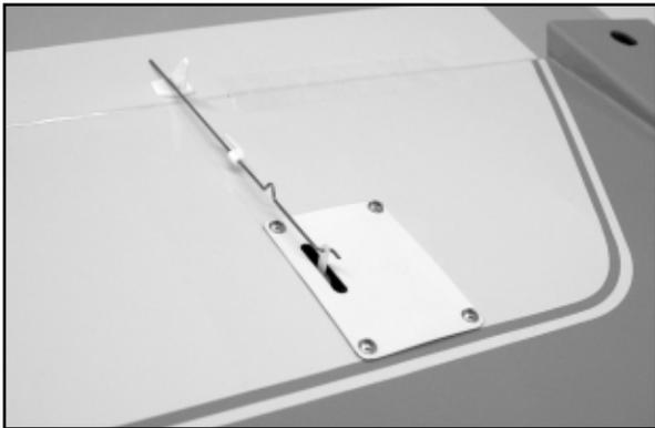
c) Hold the pushrod end against the control horn, at its outermost hole location. Use a fine tipped marker to mark the pushrod wire at the control horn hole location.
