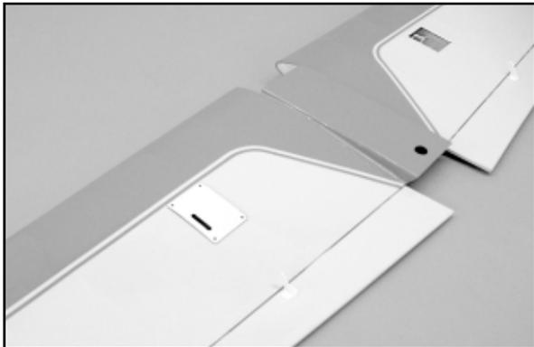
The bottom surfaces of both aileron hatch/mount covers are now lightly sanded, using 220-grit sandpaper. Move the servo output arm to position it at 90° to the servo body. Hold the aileron servo in place on the sanded side of one of the aileron hatch covers. Move the servo to center the servo arm within the slot, leaving equal clearance on both sides, as shown. This is the position that the servo is mounted.
