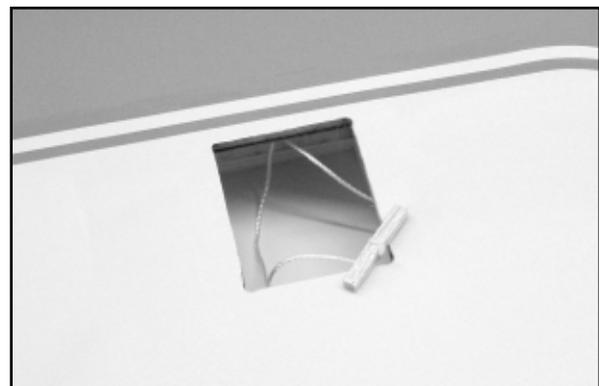
Once the string is loose, remove the scrap balsa piece. Carefully tie and tape the aileron servo lead to the end of the string.
