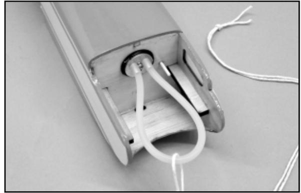
□ 2) The balsa Fuel Tank Retainer is now installed at the back of the tank, between the two fuselage side doublers. Press the retainer firmly in place against the back of the fuel tank. Use thin CA glue with an applicator tip to apply a drop or two of glue to each side of the retainer where it contacts the fuselage sides - this will secure it firmly and also allows it to be easily removed if ever necessary.
