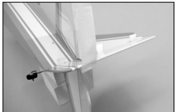
in position to the opposite side, against the elevators. As before, apply 3 or 4 drops of thin CA glue to each exposed hinge edge. Remove the tape and return the rudder to its neutral position. Allow about 10 minutes for the glue to fully wick its way through the surface of each hinge. Flex the rudder firmly in both directions to free up its movement.
