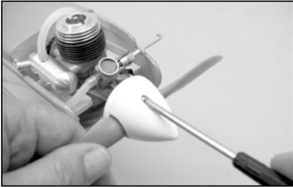
□ 5) The Norvel™ .074 engine has an exhaust outlet that can be positioned to any desired angle. We positioned ours to aim the exhaust directly out of the right side of the fuselage and then added a short length of large diameter fuel tubing to carry the exhaust past the fuselage side. In actual practice, this works quite well in keeping much of the exhaust residue off the model.
