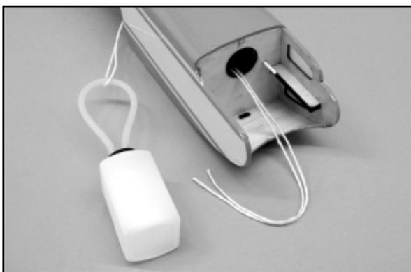
Apply a generous bead of silicon sealer (bath and tub type works well) around the stopper assembly at the front of the fuel tank. While pulling on the string from the front, guide the tank through the fuselage wing saddle and into the tank former. Continue pulling the string until the stopper assembly fits into the round cut
