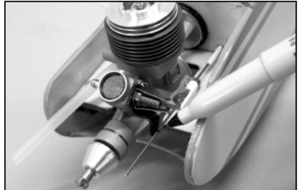
Use a pair of needle nose pliers to make a 90° bend in the pushrod wire, at the mark just made. Trim the bent end of the wire to about 3/16". Slip the bent end into the bottom hole in the throttle lever and slide the pushrod retainer forward. Lift the retainer arm over the end of the pushrod wire and press it in place.
