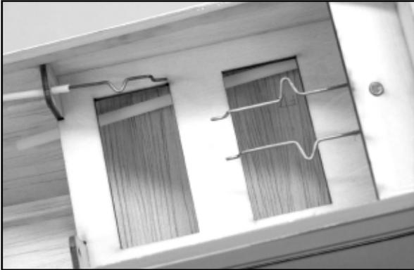
The rudder, elevator, and throttle servos are now installed onto the fuselage servo tray, as shown. We installed the rear rudder and elevator servos first and the throttle servo last. We also found it helpful to first label the servo connectors for later identification when connecting them to the receiver. As shown, position each servo's output arm to approximately line-up with the appropriate pushrod. Install the servos using the mounting screws that came with them.
