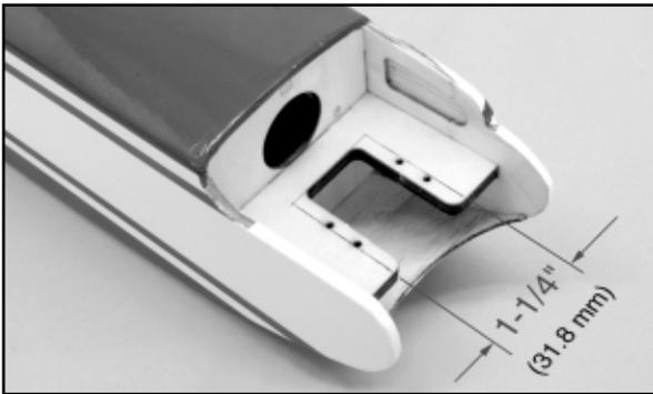
2) Hold the bottom half of the Clam Shell Motor Mount in place on the plywood plate while you mark the locations of the four new mounting holes that are needed in the plywood.
